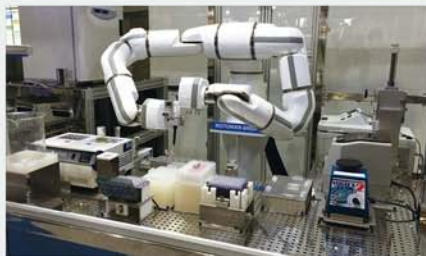
Robot performing bioanalysis for new drug development (Photo courtesy of Yaskawa Electric Taiwan Corporation)
